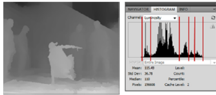
Fig. 2. The separation of a depth map into depth planes by depth thresholds (colored in red)
