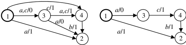
Fig. 2. Constructing a preamble for state 2
