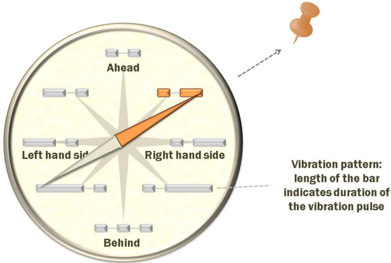
**Fig. 2.** The pointing direction is encoded in the relative length of two pulses. In this illustration the geographic reference point is somewhat to the right-hand side, so the first pulse remains short while the length of the second pulse is slightly increased.
