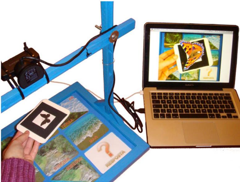
**Fig. 1.** The developed system, when used in a LCD display configuration
