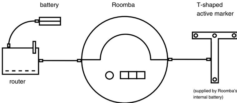
Fig. 1. Design of the hardware on the slave robot
