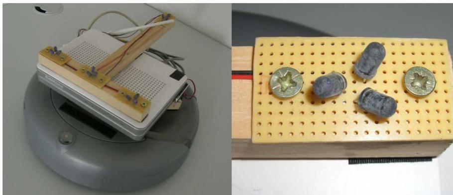
**Fig. 2.** Modified Roomba (left), One out of four infra-red LED groups (right)
