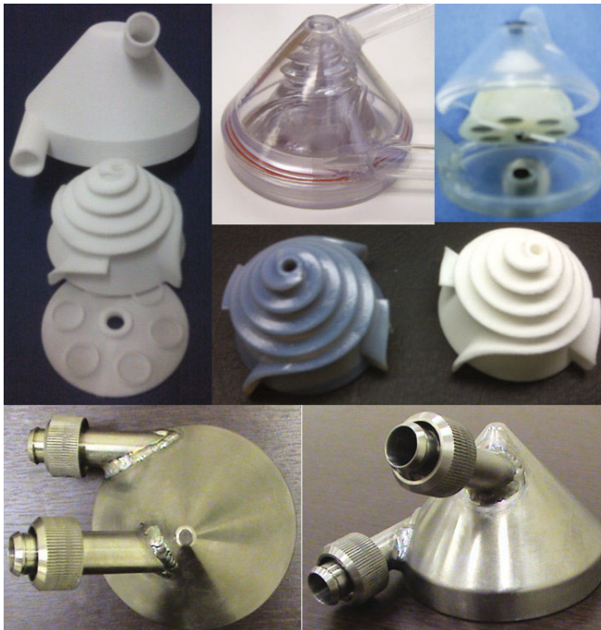
Fig. 3. Different types of prototypes obtained by SLS or Machined in different types of materials from translucent polymers to titanium
