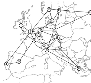
Fig. 5. European COST 239 Network (19 nodes, 37 bidirectional links)
