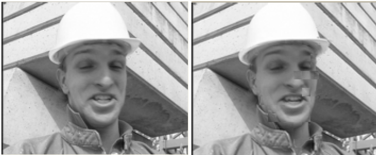
Fig. 3. Original 180th frame (left) and side information generated (right) in decoder (assumption of linear motion is not satisfied)
