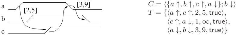
Fig. 2. A timing diagram with partial orders and its mapping into an event sequence.
