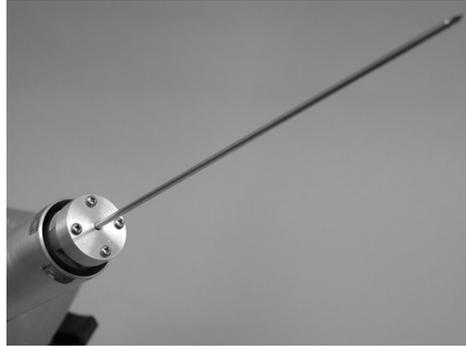
**Fig. 4.** The coaxial needle attached to the sensor.
