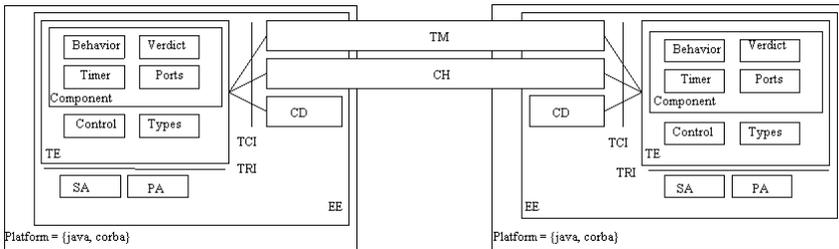
**Fig. 3.** Implementation view of a distributed TTCN-3 runtime environment. While the TTCN-3 execution environment is available on each test device (see [3]) only once, possibly distributed instances of the test management (TM) and the component handling (CH) entity exist.
