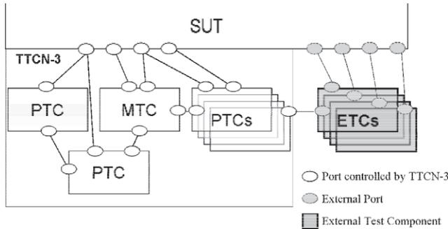
**Fig. 1.** Architecture for a test system using TTCN-3 test components (MTC – main test component and PTC – parallel test component) and external test components (ETC)
