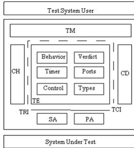
**Fig. 2.** General structure of a TTCN-3 test system as defined in TCI [3]. The test system contains the TTCN-3 executable (TE), which in turn communicates with the test management system (TM), the component handling (CH) and the coding/decoding (CD) via the TTCN-3 control interfaces. Communication with the SUT is performed using the TTCN-3 runtime interfaces (TRI), which define the interfaces between the TE and the system adapter (SA) and the platform adapter (PA).
