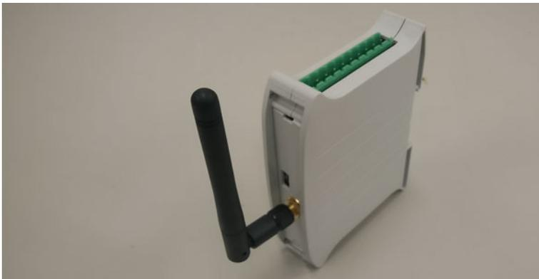
Fig. 5.14 IoT sensor node
