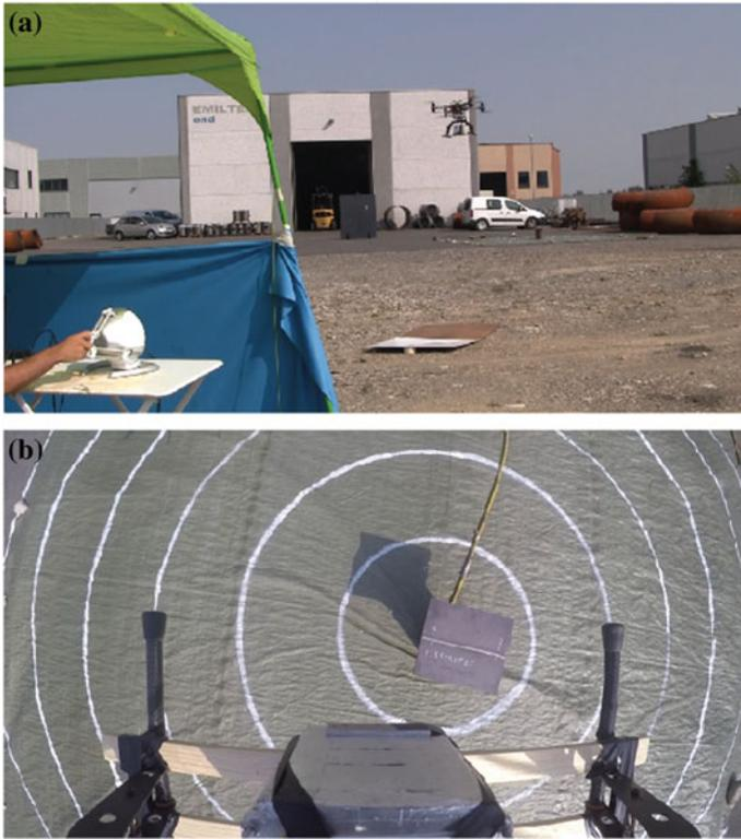
**Fig. 9.8** Localization of the nuclear source; **a** in foreground the haptic device handled by the pilot; **b** board camera image of the nuclear source
