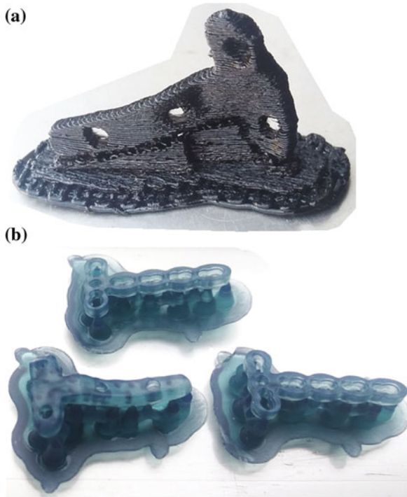
Fig. 11.6 Rolando fracture fixation plates made using FDM (a) and SLA (b)
