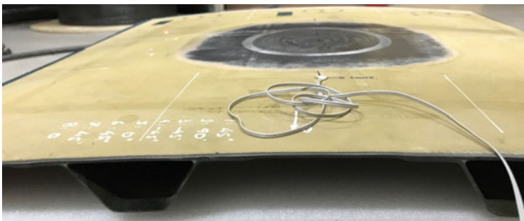
Fig. 5.41 The setup for the laser vibrometry inspection of a real CFRP panel with the scarfed and stepped areas for bonded repair
