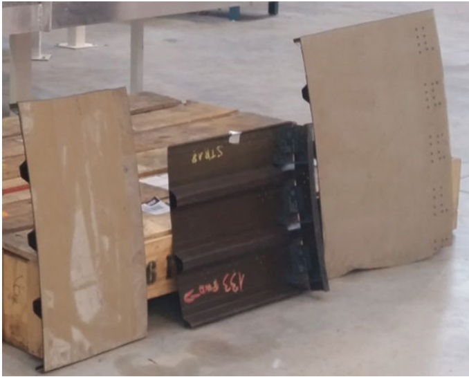
Fig. 5.4 A350 aircraft fuselage panels provided by Airbus for the demonstration of a full-scale bonded repair
