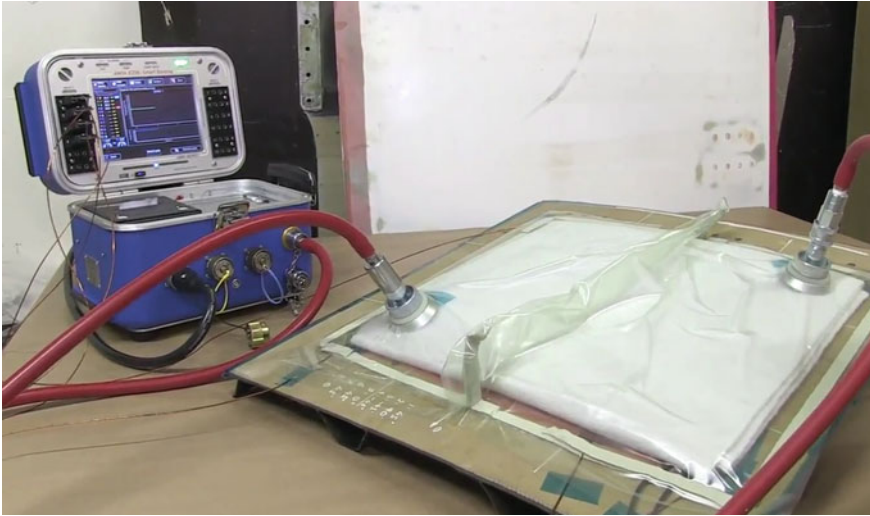
Fig. 5.13 Image taken during the full-scale demonstration of the repair process using the ANITA EZ0901 hot bonder in the ComBoNDT project
