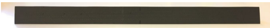
Fig. 5.16 An overview of the stringer surface after performing spot-by-spot LIBS measurements along three parallel lines, with the top, middle, and bottom lines composed of 130 analysis spots each; the left part of the specimen was contaminated, while the right part provided a clean reference surface
