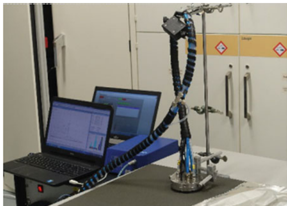
Fig. 5.20 The e-nose desorber device taking measurements on the CFRP Panel 1 within the production user case during the full-scale demonstration event
