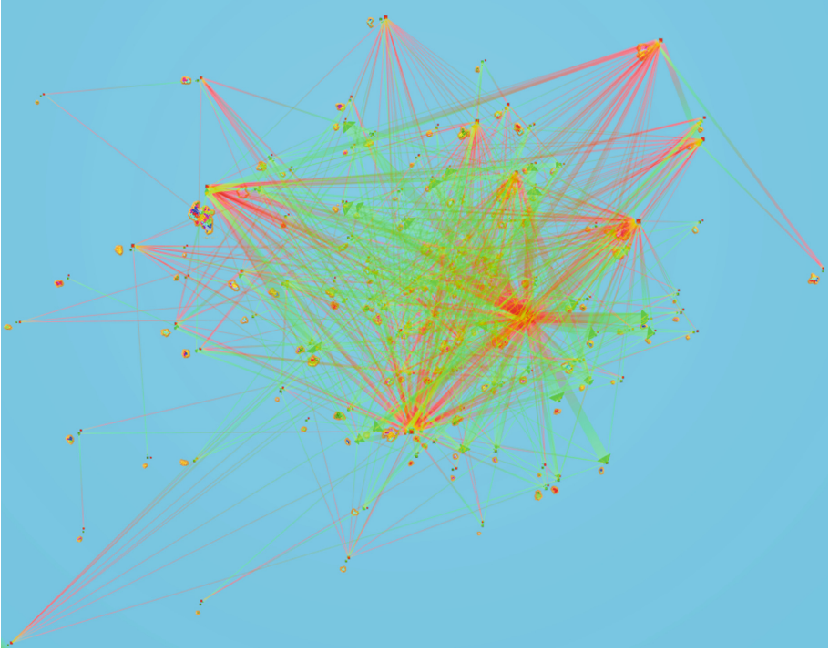
Fig. 4. Island placement based on the presented force-directed layout algorithm. Islands with the highest dependencies are accumulated in the middle, while independent islands are pushed outwards.
