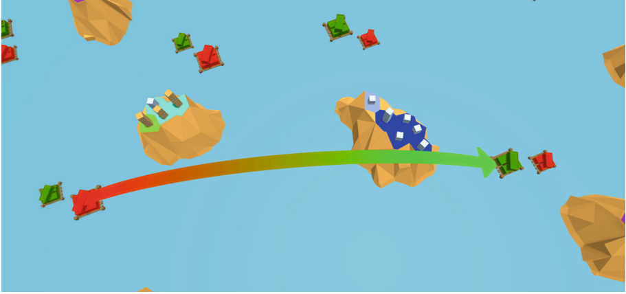
Fig. 3. Explicit dependency visualization via an arced arrow. The island on the right imports packages from the bundle on the left.
