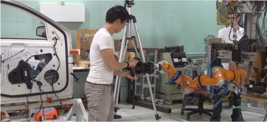
**Fig. 14.1** The robot-assistant supporting the activities of a worker performing a simulated car door assembly task
