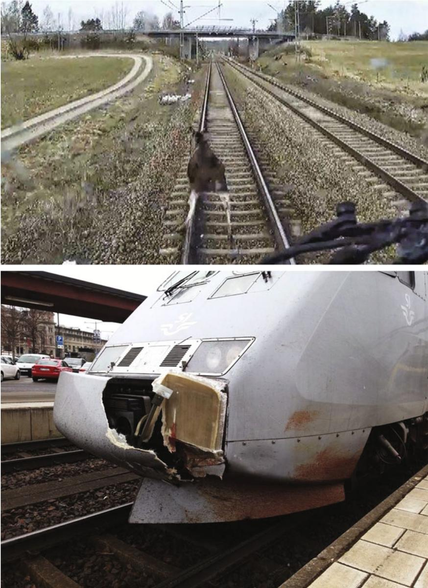
**Fig. 17.4** Train driver's view of a fleeing moose shortly before collision (above). The picture was taken with a video dashcam mounted inside the driver's cabin. The damaged front of the X2000 train engine after the moose collision (below) (*photos Jimmy Nilsson, Swedish Railways*)
