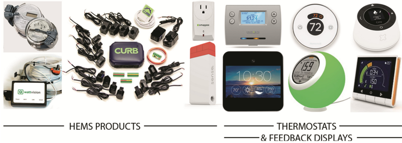
Fig. 1. Some sampled HEMS hardware (Blue Line Innovations, Wattvision, Curb, Smappee, Sense), thermostats (Energate, Lyric, Cosy) and feedback displays (Sentri, Energy Orb, Minim)
