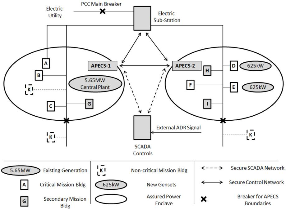
Figure 1. Conceptual architecture of a SNAPE microgrid.
