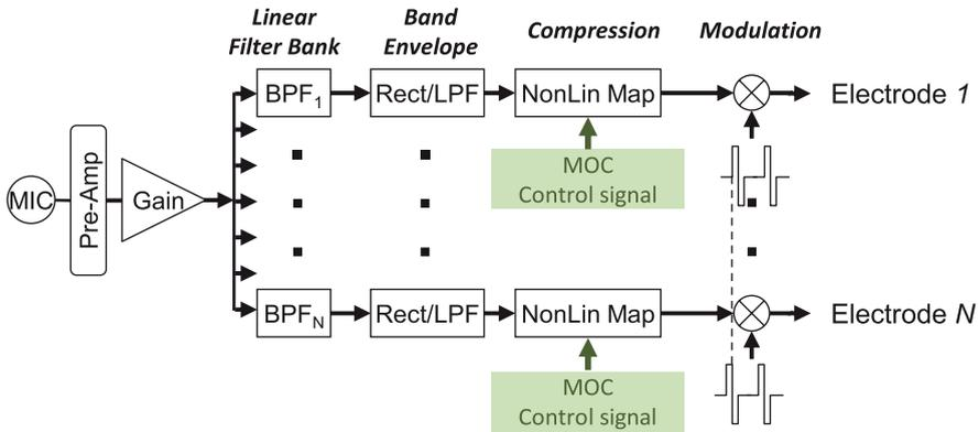
**Fig. 1** Envisaged way of incorporating MOC efferent control to a standard pulsatile CI sound processor. The elements of the standard sound processor are depicted in *black* (Wilson et al. 1991) and the MOC efferent control in *green*. See the main text for details
