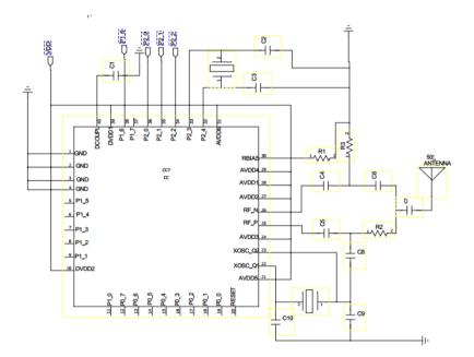
Fig. 6. Application of CC2530 circuit
