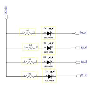
Fig. 8. Principle diagram of LED alarm
