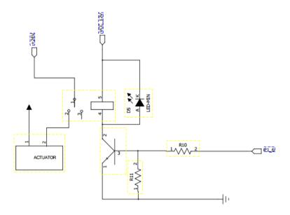
Fig. 7. Principle diagram of relay driver
