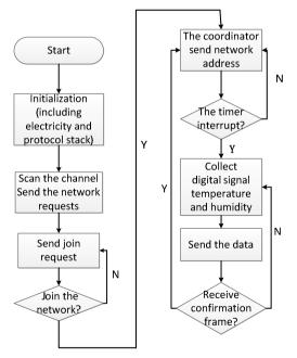
Fig. 10. Flow chart of acquisition node
