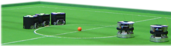
Fig. 1. Small size league robots facing against each other at the start of a game with orange golf ball at the center of green carpeted field (Color figure online).
