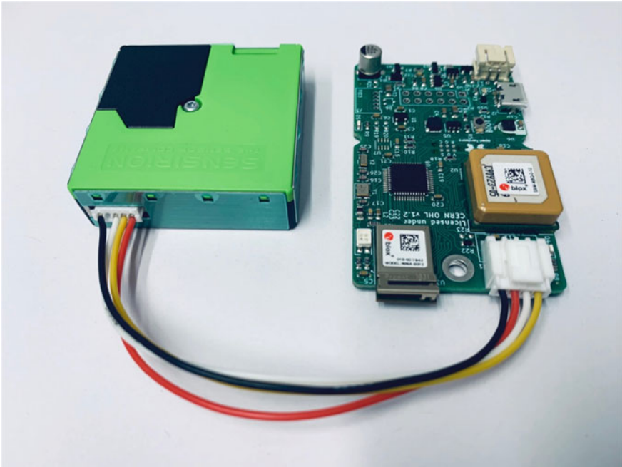
Fig. 1 Air quality sensor produced within the FuturICT 2.0 City Cup setting
