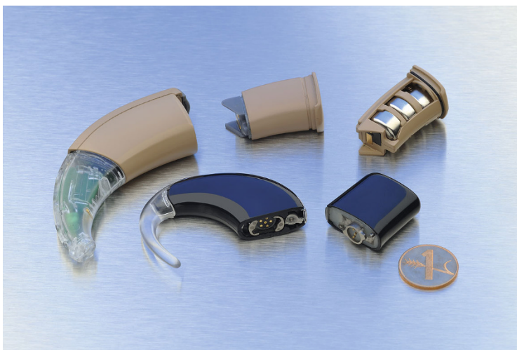
Exhibit 26.31 Wyon battery system
