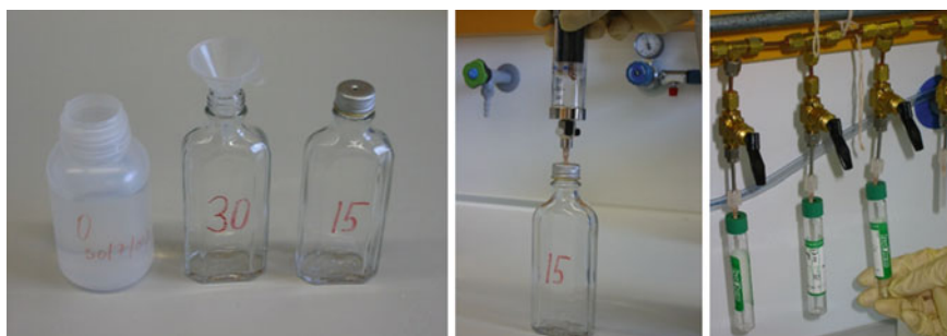
Plate 7.3 Soil extracts are transferred to medical flasks for conversion of \text{NO}_2^- and \text{NO}_3^- to \text{N}_2\text{O} ; gas samples are taken through the septa with syringes and then are transferred to pre-evacuated exainers (from left to right)
