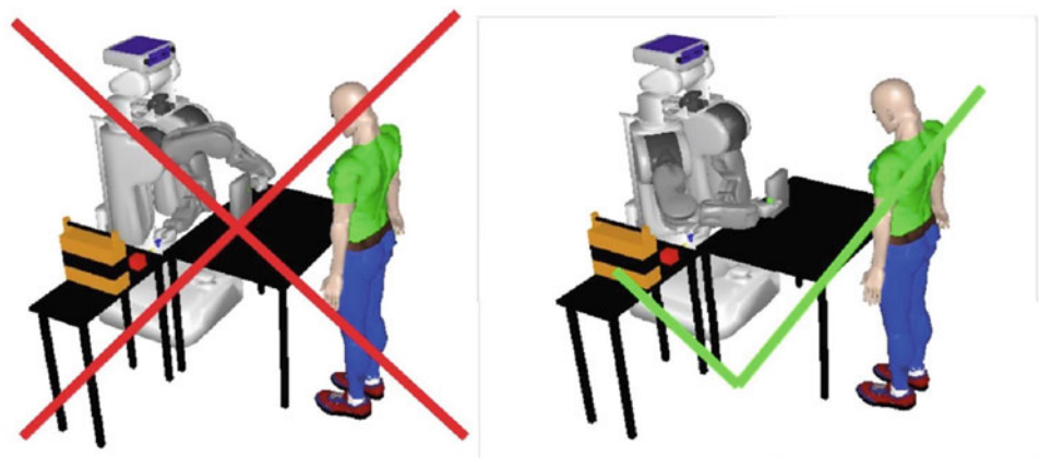
Fig. 4 Two final positions of the arm of the robot to get the object. The one at right is better from an interaction point of view since it is easily understandable by the human. However, from a computational point of view (and even from an efficiency if we just consider the robot action that needs to be performed) they are equivalent. Consequently, we need to take these features explicitly into account when planning robot motions. That is what human-aware motion planning aims to achieve. Copyright laas/cnrs https://homepages.laas.fr/acloedic
