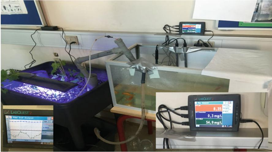
**Fig. 23.1** The aquaponic learning and experimental mock-up. The illustration shows the setup including aquarium fish tank and the monitoring devices that are used to measure the equilibrium of the whole system. The last part is the core of the learning goal for students. (Pictures: courtesy of Lija Gunnarsdottir)
