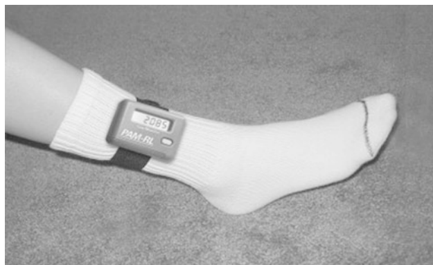
Fig. 39.12 Example of a high-precision activity monitor worn on the ankle to detect leg movements
