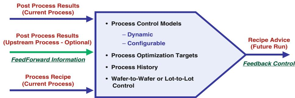
**Fig. 1** Input/output structure of a typical R2R control solution
