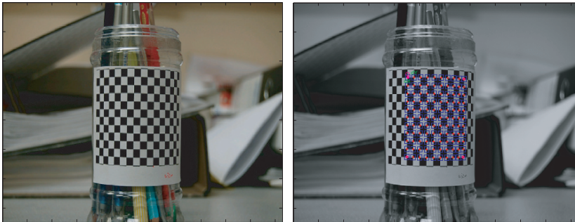
Fig. 11.12 Object image (left) and image with extracted corners (right)
