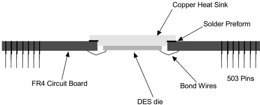
**Fig. 4.** Cross Section of the 503-Pin Package
