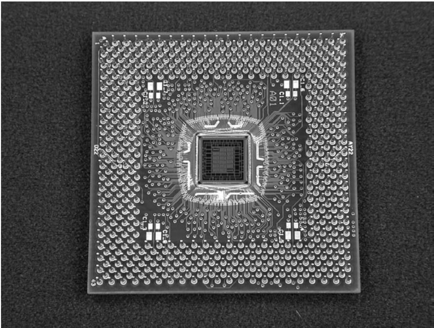
**Fig. 5.** Picture of the 503-Pin FR4 Board Package
