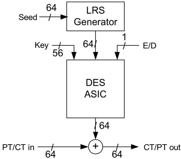
Fig. 6. Encryption/Decryption for Counter Mode
