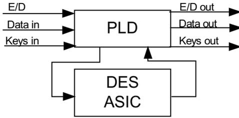
**Fig. 8.** Iterative, Single ASIC, Triple DES Implementation
