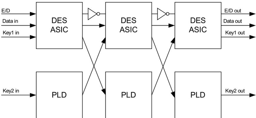
Fig. 7. Cascaded, Multiple ASIC, Two Key, Triple DES Implementation
