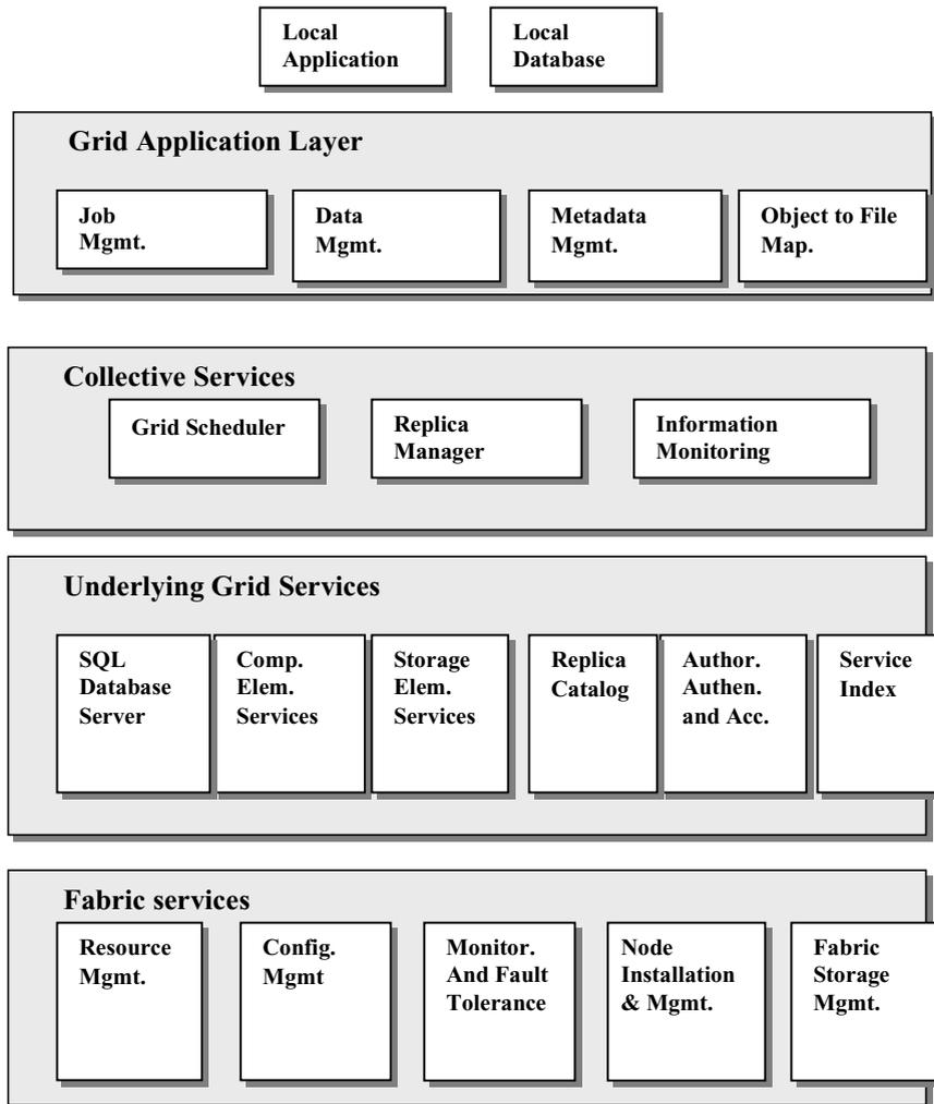
Fig. 2. The detailed multi layered EDG GRID architecture
