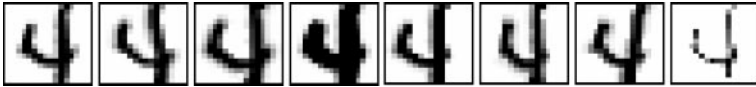
Fig. 2. Example of first-order approximation of affine transformations and line thickness. (Left to right: original image, diagonal deformation, scale, line thickness increase, shift left, axis deformation, line thickness decrease)
