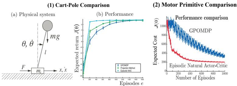
**Fig. 2.** This figure shows two comparisons, (1) cart-pole and (2) motor primitive learning. The physical set-up of a cart-pole balancing is shown in (1.a), and in (1.b) the performance of GPOMDP, the projection natural gradient, and the Episodic Natural Actor-Critic in comparison. The latter clearly outperforms the first two.
