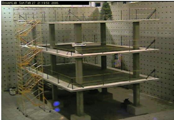
**Fig. 6.** Image of the test structure (30 × 50 × 35 feet) at the Bowen Lab for Structural Engineering at Purdue University. The structure will be subject to a variety of external loads and responses will be used to validate model reduction and simulation frameworks. A live web-cam image of this structure is posted at [http://newton.ecn.purdue.edu/ ce/Bowen/Webcam/](http://newton.ecn.purdue.edu/ce/Bowen/Webcam/)
