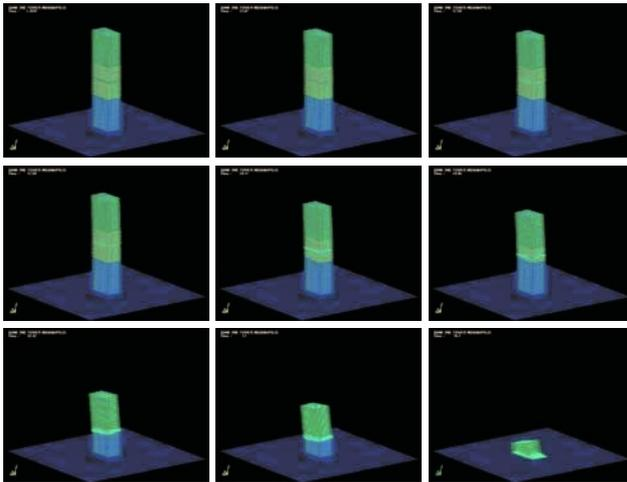
**Fig. 3.** Simulation of heat-induced structural failure – a fire on the 25th floor of the Bank-One tower in downtown Indianapolis is simulated using a coupled fire-structure code (wireframe model shown here). The entire simulation is available at <http://www.cs.purdue.edu/homes/ayg/SIM>
