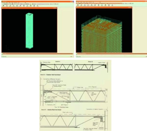
**Fig. 5.** A high-resolution mesh of the World Trade Center (WTC), developed using detailed blueprints (of the kind shown in bottom panel), which will be used for high-fidelity coupled fire-structure simulation of the WTC collapse
