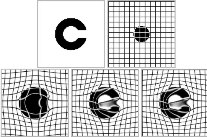
**Fig. 1.** Registration of a disk on a C. The grids are added after the registration to help visualizing the deformation. **Top:** reference image on the left, and image to register on the right. **Bottom:** from left to right, registration results with demons ( $\sigma = 1.2$ ), with the new method simulating elastic deformations ( $\sigma_{fl} = 0$ ,  $\sigma_{el} = 1.2$ ) and with the new method simulating fluid deformations ( $\sigma_{fl} = 3$ ,  $\sigma_{el} = 0$ ).
