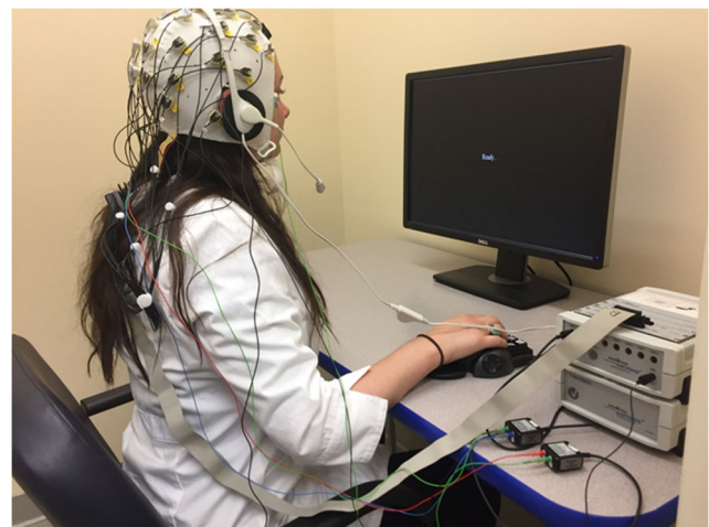
Fig. 2 Example of the S-1 Voice Key device used to collect digitized time stamps of response times of cued recall for semantic associates in the current study, concurrent with EEG recordings
