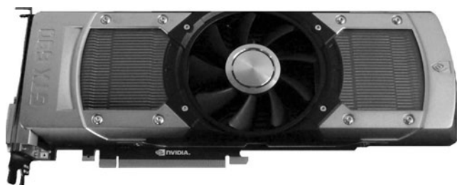
Fig. 1 The Nvidia GTX 690 graphics card, containing two GPUs and a total of 3,072 processor cores
