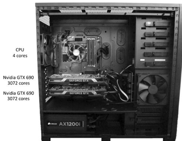
Fig. 2 The physical location of a CPU and two graphics cards in an ordinary PC. By using two Nvidia GTX 690 graphics cards, the user gets a PC equipped with 6,144 processor cores at the price of about $3,000
