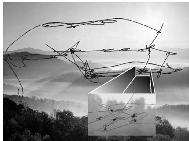
Figure 1. Example of oculomotor activity during unconstrained viewing of a natural scene. A trace of eye movements recorded by a dual-Purkinje-image eyetracker is shown superimposed on the original image. The inset panel shows an enlarged portion of the trace in which small fixational eye movements are present. The image was examined for a period of 30 sec.
