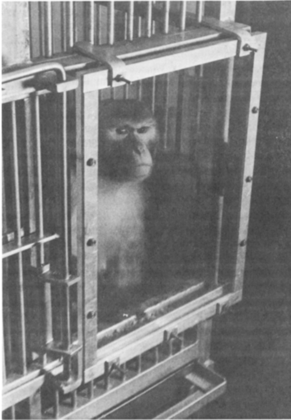
Fig. 4. The second type of window fits over a sliding—rather than hinged—access door of a home cage. An adult male rhesus macaque is shown within.
