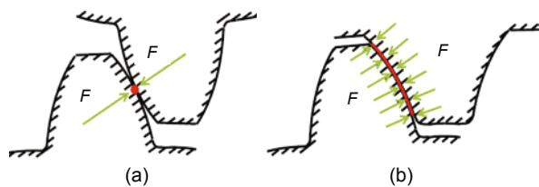
Fig. 1 Contact in gear teeth (a) and spline coupling teeth (b)
