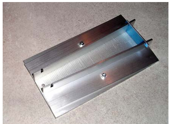
Fig. 1 Photo of support configuration (support elements riveted to support base plate) used for cyclic mechanical movement of sealant
