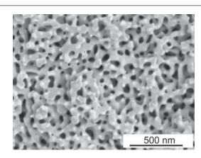
Figure 1. Representative image of nanoporous gold. Reproduced with permission from Reference 28. © 2005 Cambridge University Press.
