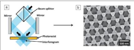
Figure 5. (a) Schematic of multibeam interference lithography and (b) representative scanning electron microscope image of a 3D polydimethylsiloxane/air phononic crystal structure fabricated via interference lithography template. (a) Reproduced with permission from Reference 63. © 2012 Wiley-VCH. (b) Reproduced with permission from Reference 74. © 2006 American Chemical Society.
