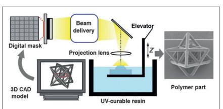
Figure 3. Representative image of a microlattice fabricated by projection microstereolithography, a layer-by-layer technique capable of fabricating arbitrary, microscale, 3D structures with a resolution of ~5 mm. Note: CAD, computer-assisted design. Reproduced with permission from Reference 30. © 2014 American Association for the Advancement of
