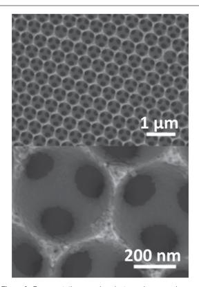
Figure 6. Representative scanning electron microscope images at different magnifications of nanocrystalline silicon inverse opals templated from 480-nm silica spheres for use as negative electrodes in lithium-ion batteries. Reproduced with permission from Reference 81. © 2009 Wiley-VCH.
