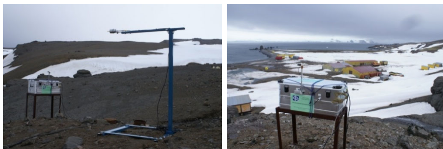
Fig. 3. Photographs of the electric field sensor and data acquisition system at Arctowski station, installed there in December 2012. Photography by Sylwia Łukawska.
