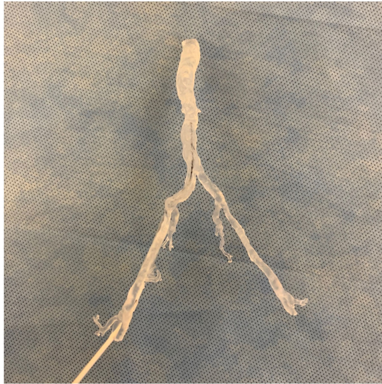
Fig. 2 3D printed aortic vasculature from the 40 keV VMI data at 25% scale size. The model was printed using the Formlabs Form 2 SLA 3D printer with standard clear resin material. A guide wire is placed through the right common femoral artery simulating vascular access
