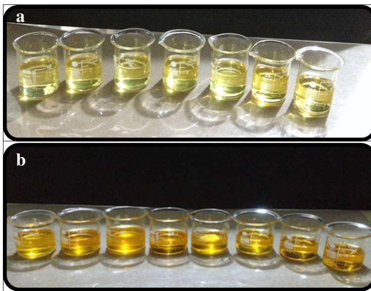
Fig. 7 Results of dye test; upper picture (a) representing candesartan cilexetil nanoemulsion formulations before adding methyl orange dye (water soluble) and the lower picture (b) showing the homogenous miscibility of the dye with nanoemulsions
