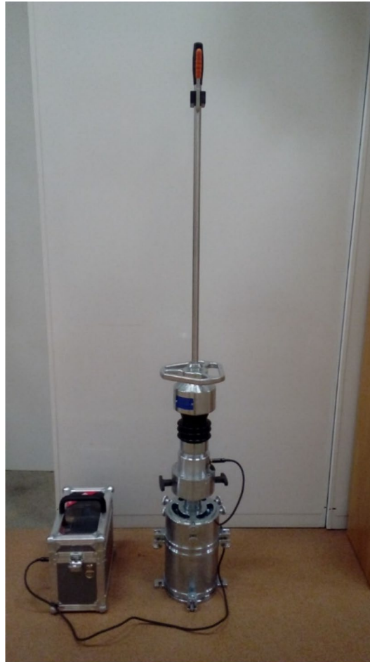
Fig. 2 Laboratory dynamic CBR test on sandy CBR soil samples prepared using modified compaction method
