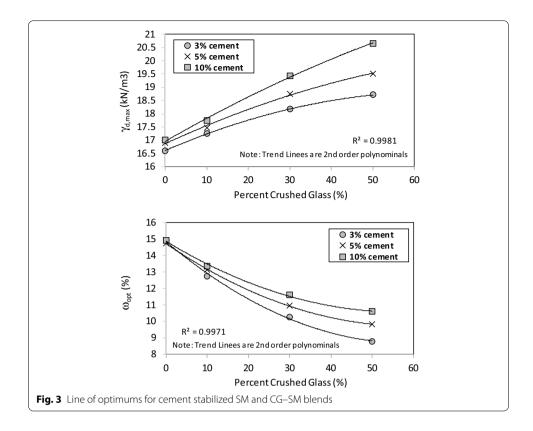
showed that the CG-SP blends were denser than the individual material. Also, during the compaction tests, it is probable to crushed the CG under hammer load. Associated this subject in laboratory, it was revealed that the amount of particles crushable due to compaction test was negligible (around 2%).
