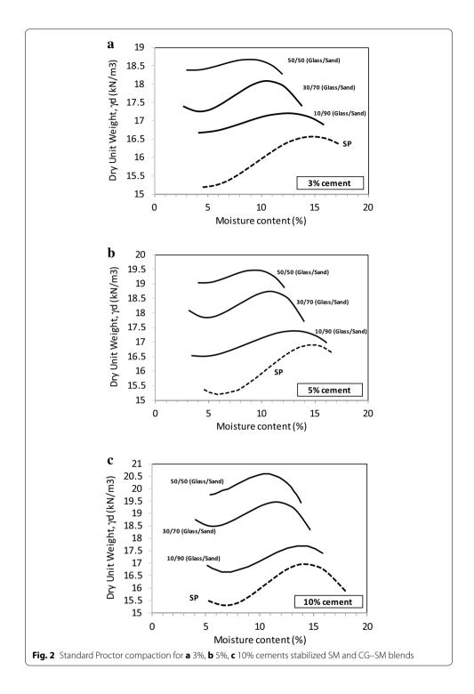
For example, increasing in the amount of cement from 3 to 10% could contribute to increase in the sandy soil  $\gamma_{d,max}$  from 16.6 to 18.71 kN/m³ (about 3%). While this proportion of cement, Addition of the crushed glass in mixed 50% CG–SP will increase amount  $\gamma_{d,max}$  from 18.71 to 20.66 kN/m³ (approximately 11%).Therefore, (as shown in Fig. 3) the values of  $\gamma_{d,max}$  increased in a nearly linear fashion with CG increment, which
