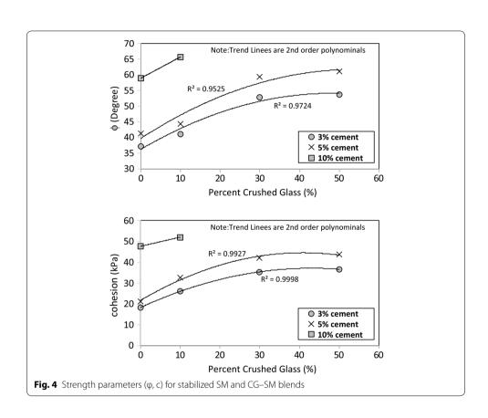
stabilized SP increased significantly as the percentage of CG increased. Considering that CG aggregates have sharp corners, by addition of CG, fastening between aggregates grew up, and the adhesion between the aggregates may also increase the shear resistance.
