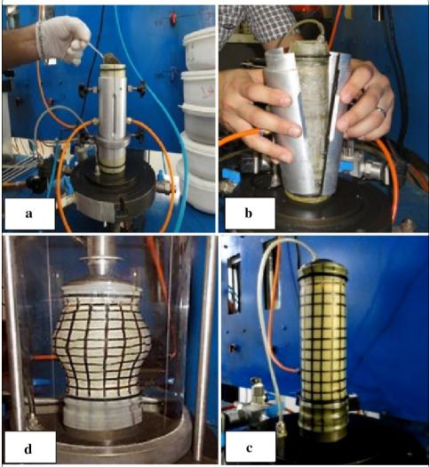
**Fig. 6** The process of sample preparation (**a**) pouring sand into mold, (**b**) open the mold and applying suction to sample maintenance, (**c**) prepare samples for testing and (**d**) at the end of the test specimens deformed
