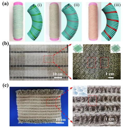
**Fig. 5** a Composite yarns prepared from varied colored polyester filaments. Optical images of the woven textiles designed with **b** different patterns and **c** stereo visual effects
