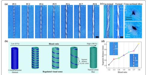
**Fig. 2** a Optical images of the composite yarns prepared with varied blend ratios. **b** Schematic illustration of the blend ratios induced structural changes and regulated visual sense. **c** Optical observations of the segmented structure at different twisted states and regions. **d** Segment distance as a function of bending ratios
